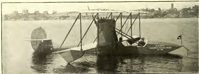
A Burgess Flying Boat (70-h.p. Renault engine) supplied to the U.S. Navy. For description see page 560.
